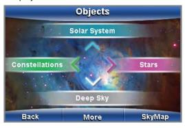
Notice the "Solar System" option is at the top of the screen. Press the UP ARROW to select "Solar System". The Solar System screen displays.
